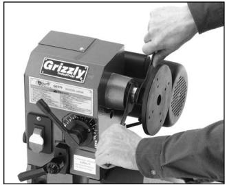
Figure 10. Attaching the faceplate.
